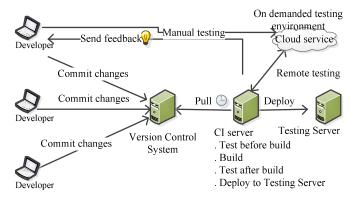
Fig. 1. A CI components in modern client-side web application
