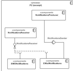
Figure 3.3.: Excerpt of the Component Diagram for the Motivating Example
