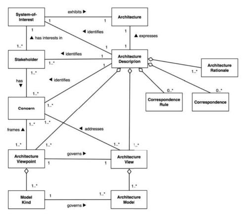
Figure 2.1.: The Meta-Model of an Architecture Description [420]
