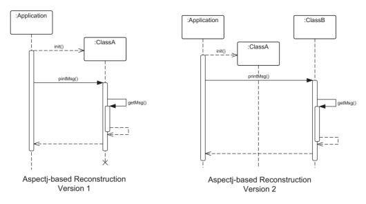
Figure A.3.: Demonstrating Polymorphism Anomaly - Reconstructed Sequence Diagrams using AspectJ
