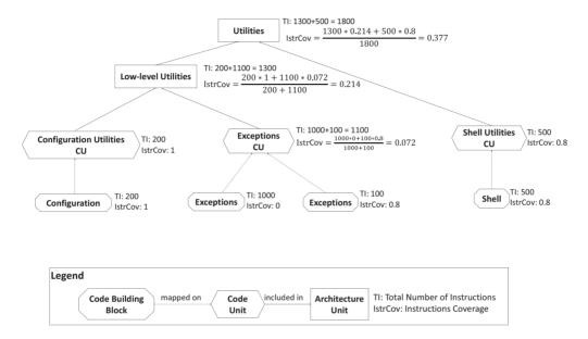
Figure 8.4.: Computation of Instructions Coverage on the for Code- and Architecture Units Level
