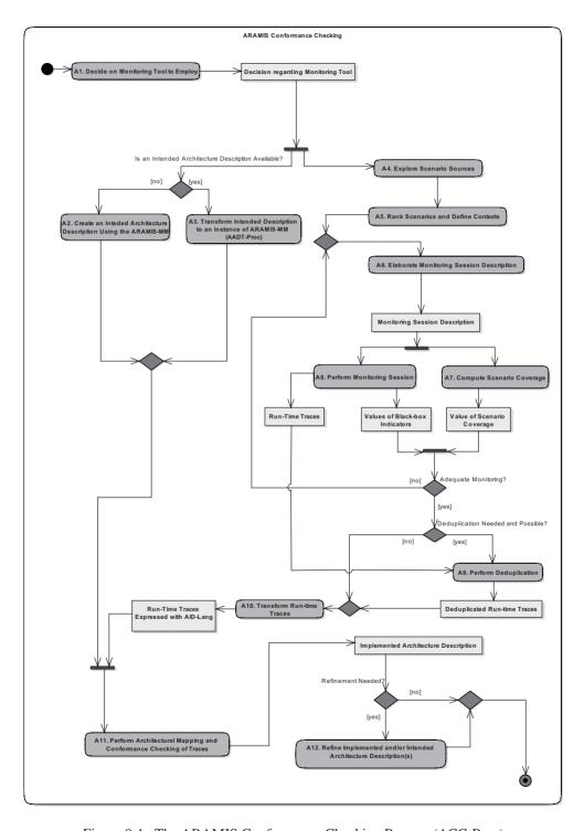
Figure 9.4.: The ARAMIS Conformance Checking Process (ACC-Proc)
