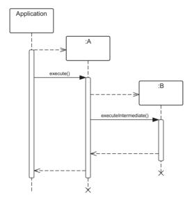
Figure A.8.: The Partial Trace Anomaly - Sequence Diagram based on Dynatrace and Kieker Monitoings when the Chain End is Un-instrumented
