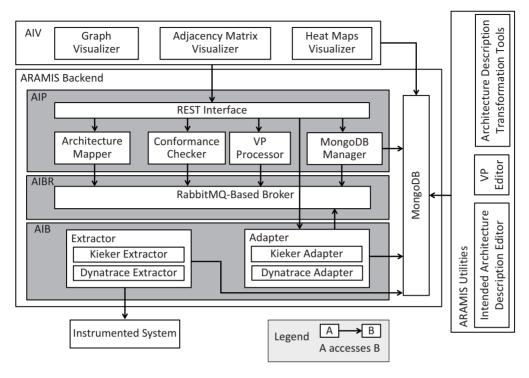
Figure 10.2.: The Intended Architecture of the ARAMIS Toolbox
