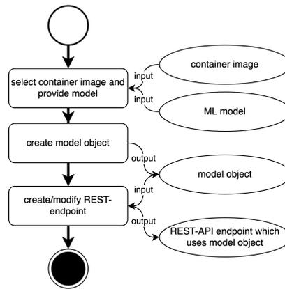
Figure 3: Graphical representation of the deployment process on Amazon's SageMaker
