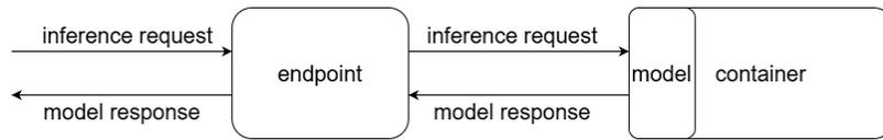
Figure 7: General deployment pattern of the three analyzed tools
