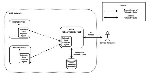
Figure 5.8.: Telemetry data collection from deployed microservices using an MSA Observability tool to comprehend their run time behaviour.
