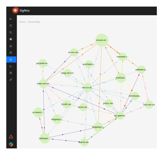
Figure 8.3.: Service map view of E-commerce application showing communication between microservices when receiving API requests.
