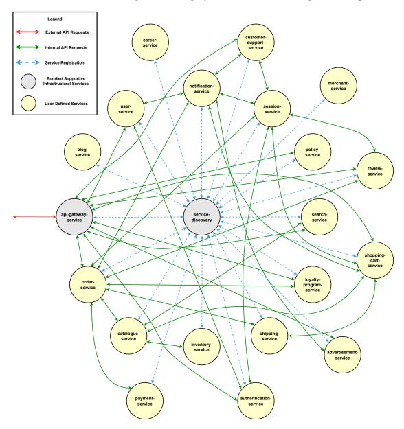
Figure 7.3.: Envisioned architectural view of the modelled E-commerce microservice application illustrating various microservice interactions.
