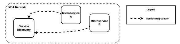
Figure 5.5.: Self-registration service discovery design pattern allows services to register with the service registry and be discoverable in MSAs.
