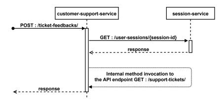
Figure A.12.: Message sequence model illustrating the functional requirement to provide feedback to customer support (FR15).
