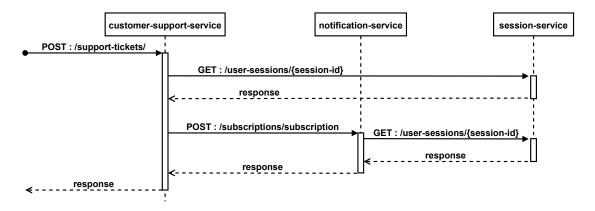
Figure A.11.: Message sequence model illustrating the functional requirement to create customer-support tickets (FR14).
