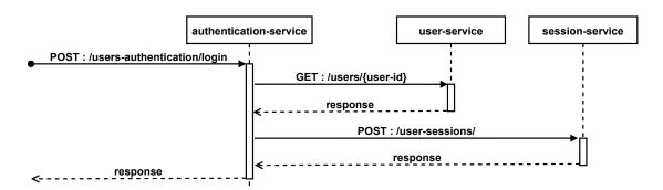
Figure A.2.: Message sequence model illustrating the login functional requirement (FR3).
