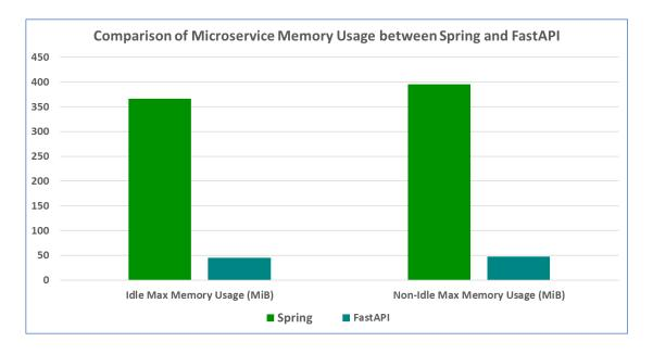
Figure 8.8.: Memory usage comparison between Spring and FastAPI microservices.
