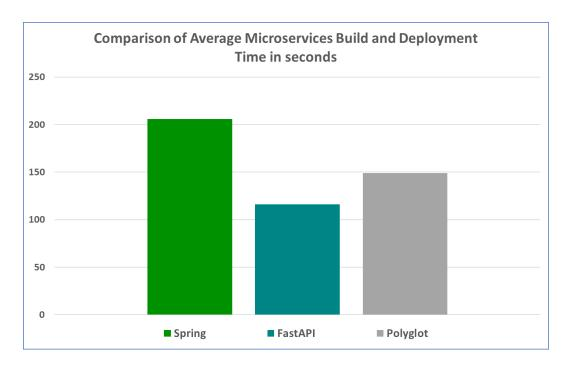
Figure 8.5.: Comparison of average microservice build and deployment time for Spring, FastAPI and Polyglot generation scenarios.
