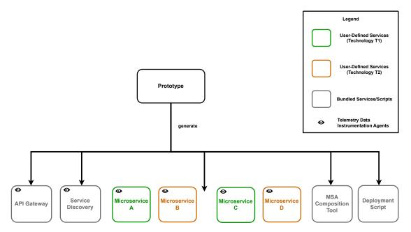
Figure 4.4.: Generation of various types of microservices by the prototype after parsing the MAPI-DM input.
