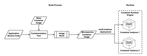
Figure 5.7.: Service instance per container design pattern to have isolated service deployment.
