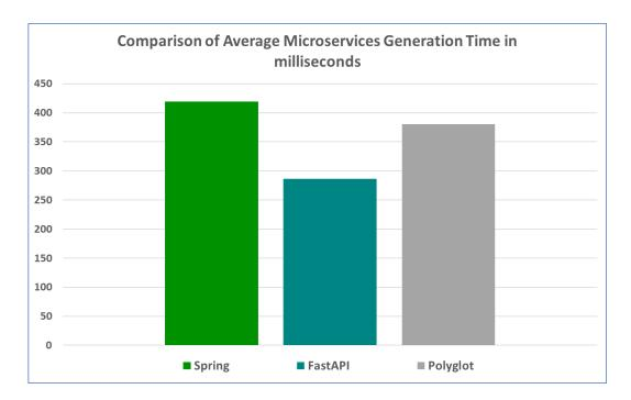
Figure 8.4.: Comparison of average microservice generation time for Spring, FastAPI and Polyglot generation scenarios.
