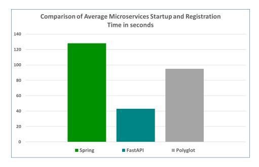
Figure 8.6.: Comparison of average microservice startup and registration time for Spring, FastAPI and Polyglot generation scenarios.
