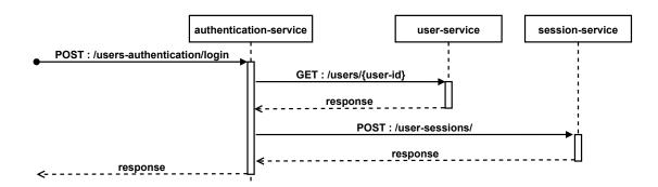
Figure 2.1.: Message sequence model illustrating the login functional requirement.
