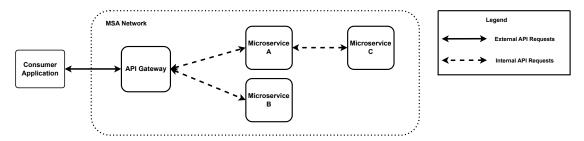
Figure 5.4.: API-Gateway design pattern offering clients a unified interface to communicate with application's microservices.
