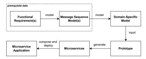
Figure 4.1.: A conceptual approach to generating microservice applications that can be used to mock MSAs.
